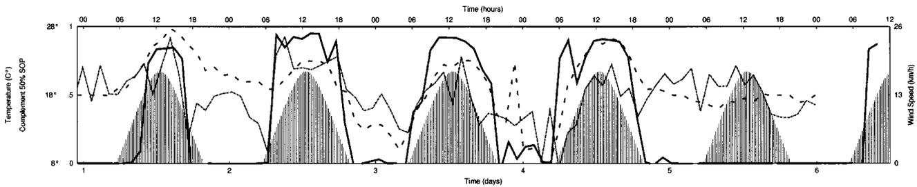
Fig. 2. Normalized complement 50% SOP autocorrelation function (dark line, a larger value corresponds to a faster changes), normalized sun altitude (parabolas), normalized temperature (dotted line), and normalized wind speed (dashed-dotted line) as a function of time in the summer.
