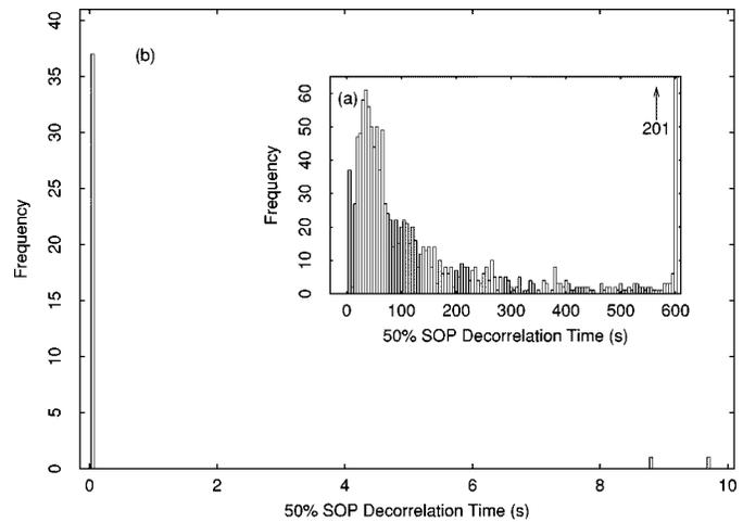
Fig. 6. (a) Histogram of 1340 Fiber II 50% SOP decorrelations (frequency as a function of time) during the winter. Bandwidth is 5 s. (b) The first 10 s of part (a). Bandwidth is 0.1 s.
