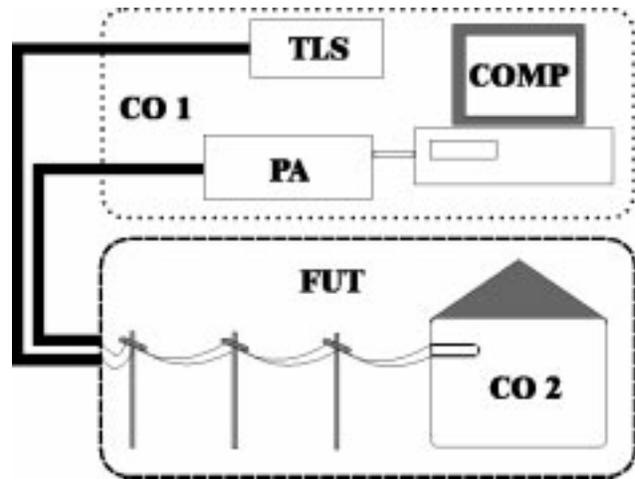
Fig. 1. Experimental setup of field fiber PMD measurement. CO1: Central office 1. TLS: Tunable laser source. PA: Polarization analyzer. COMP: Experiment control computer. FUT: Fiber under test. CO2: Central office 2.
