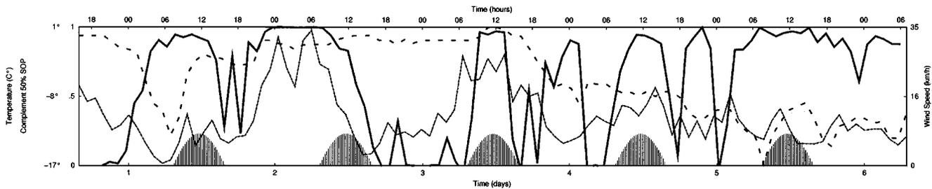
Fig. 3. Normalized complement 50% SOP autocorrelation function (dark line, a larger value corresponds to a faster changes), normalized sun altitude (parabolas), normalized temperature (dotted line), and normalized wind speed (dashed-dotted line) as a function of time in the winter.
