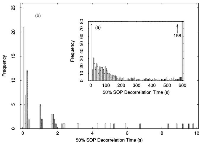
Fig. 5. (a) Histogram of 798 Fiber I 50% SOP decorrelations (frequency as a function of time) during the winter. Bandwidth is 5 s. (b) The first 10 s of part (a). Bandwidth is 0.1 s.
