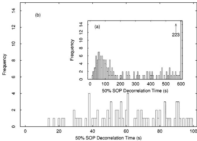
Fig. 4. (a) Histogram of 388 Fiber I 50% SOP decorrelations (frequency as a function of time) during the summer. Bandwidth is 5 s. (b) The first 100 s of part (a). Bandwidth is 1 s.
